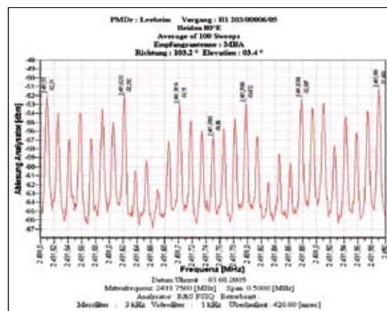
FIGURE 28 Beidou spectrum lines
