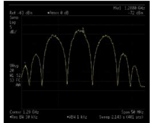
FIGURE 11 GIOVE-A E6 Measured by the Stanford Dish
