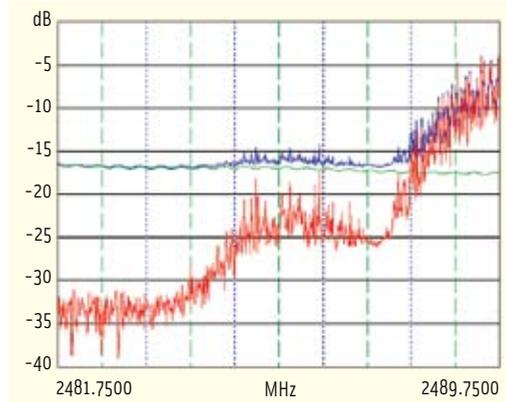
FIGURE 26 Lower first sidelobe of Beidou spectrum
