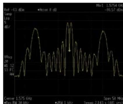
FIGURE 4 GIOVE-A E1-L1-E2 signal collected using the Stanford Dish
