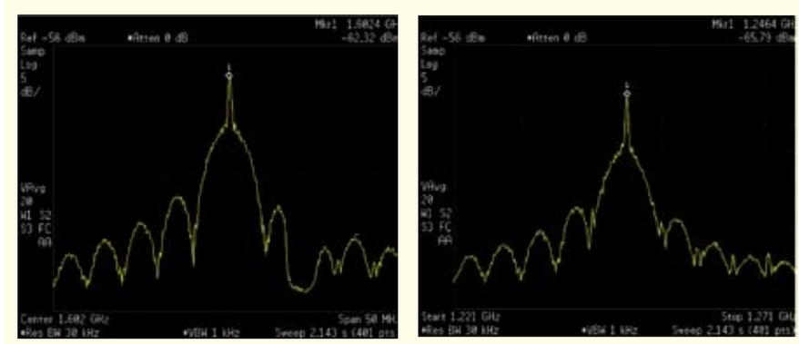
FIGURE 21 COSMOS 2404 (GLONASS 701) L1 and L2 Spectrum
