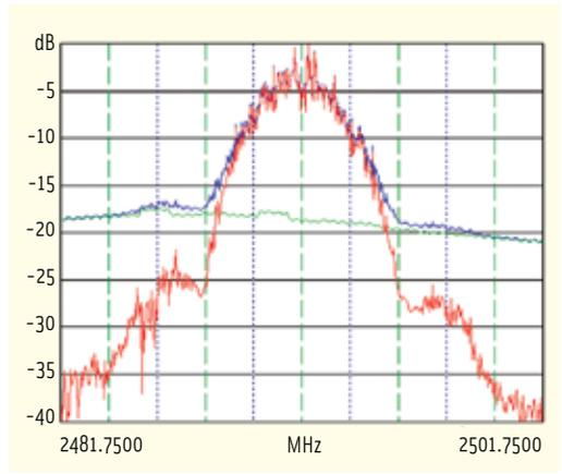
FIGURE 25 Beidou 1B measured spectrum at 2491.75 MHz
