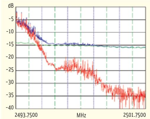
FIGURE 27 Upper first sidelobe of Beidou spectrum
