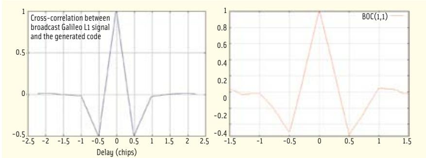
FIGURE 8 Normalized correlation function of GIOVE A BOC(1,1) modulation at L1 (Stanford (Left), CNES (Right))
