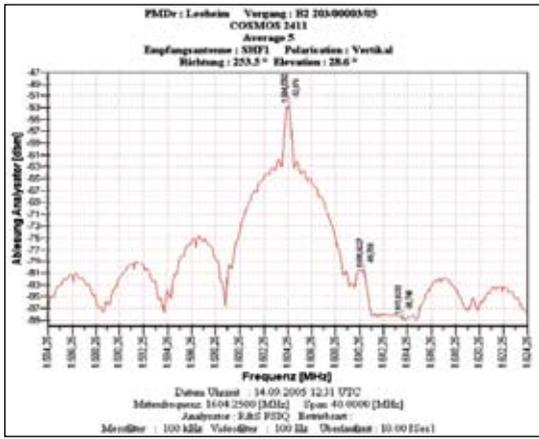
FIGURE 22 GLONASS 712 signal measured with Leeheim spectrum analyser
